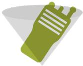
Detect the tilt or the lack of movement of a radio to generate an emergency message.
